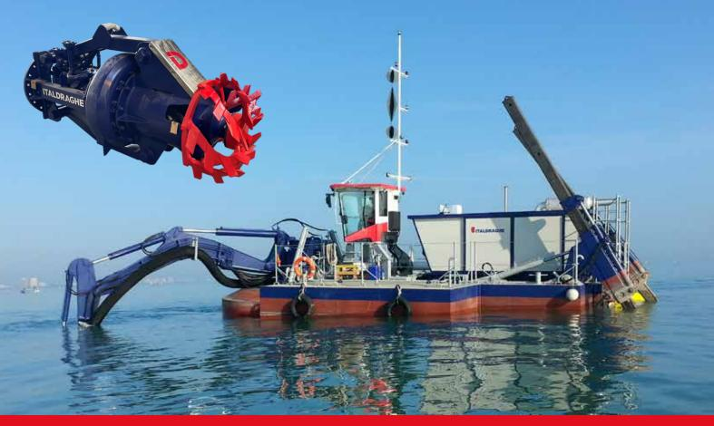
Italdraghe, based on the pluriannual experience of cutter suction dredger production, has developed the multifunctional amphibious dredger in order to perform all shallow water work from dry ground to water and marshy/muddy soils. This dredger is specifically designed for multi purposes work with only one machine – water work, for working from the land side, suction dredging, excavating, raking and pile-driving.
